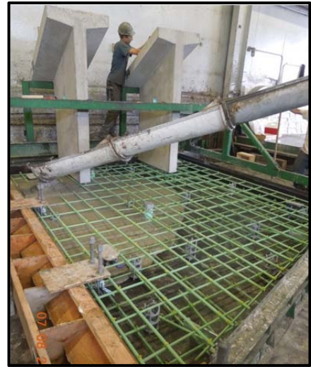
Wingwall being cast a precast plant.
