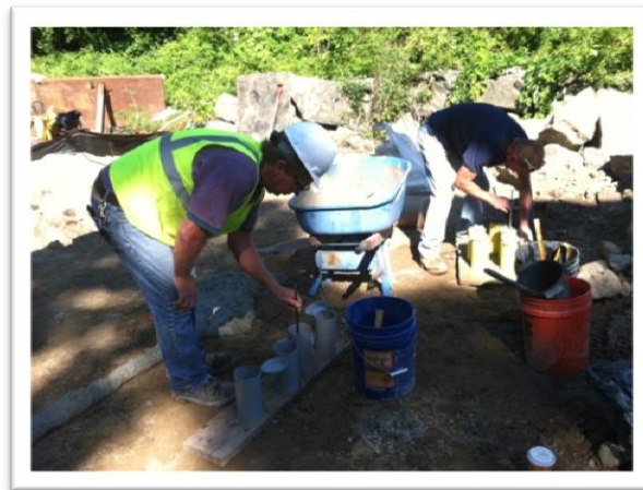
Quality Assurance Testing of Field Placed Concrete
