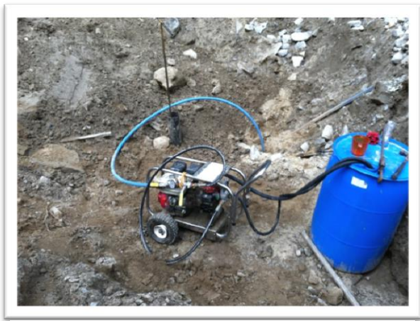
Waterline Pressure Test Apparatus
